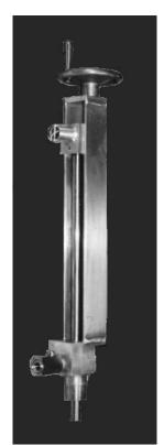
The *Model ITS* includes a stainless steel jack screw to insert and remove the temperature sensor up to 4" (100mm) into the pipe. The standard retractor housing is from aluminum although SS is also available. Bronze bushings are used to minimize lubrication requirements. Double o-ring seals are used for positive sealing. A vent valve is included for pressure release if the unit is to be removed.
